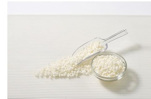
*Sample of PHA bioplastic resin pellets produced by Metabolix*
